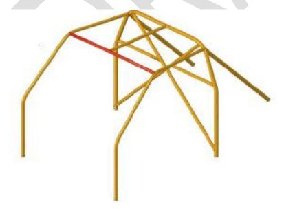
• There must be diagonal members fitted in the B pillar and shall be straight. The lower end of the diagonal shall join the main hoop or the backstay not further than 100mm from the
